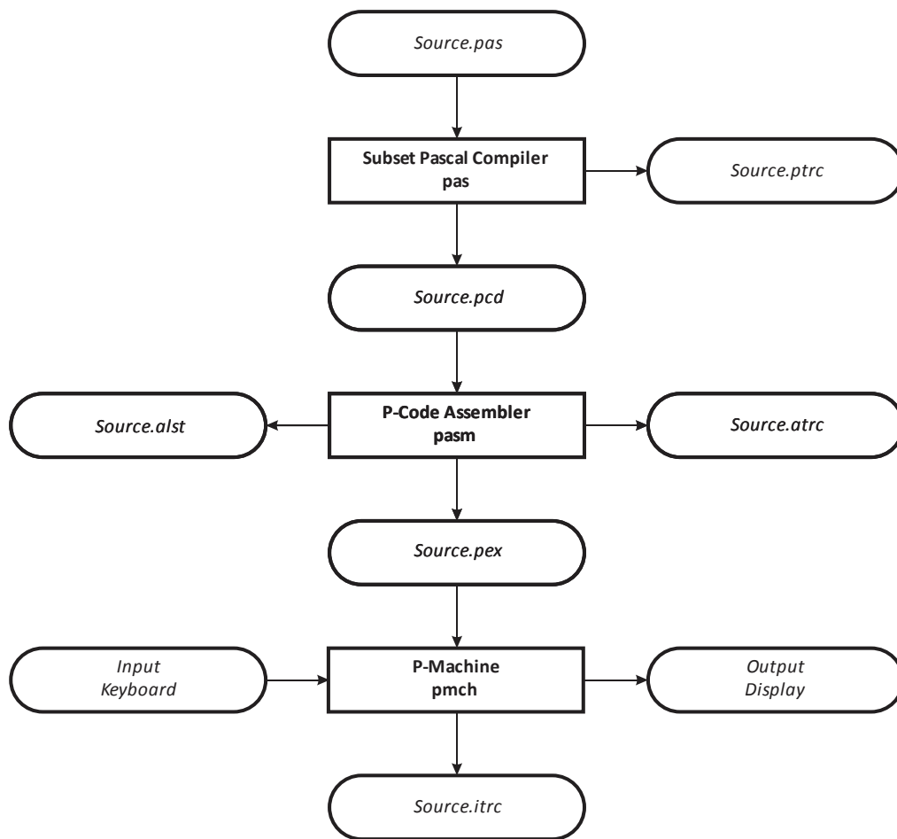
Figure 1. Subset Pascal Compiler, P-Code Assembler, and P-Code Interpreter.
