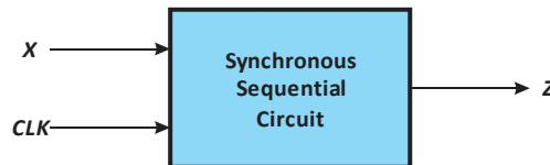
Arbitrary Synchronous Sequential Circuit Block Diagram
