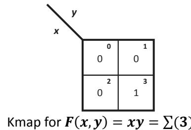
Please note that the minterm numbers – the cell numbers – are placed in the upper right of each cell. The values printed in each cell are the values of the Boolean function  $F(x, y)$ .
