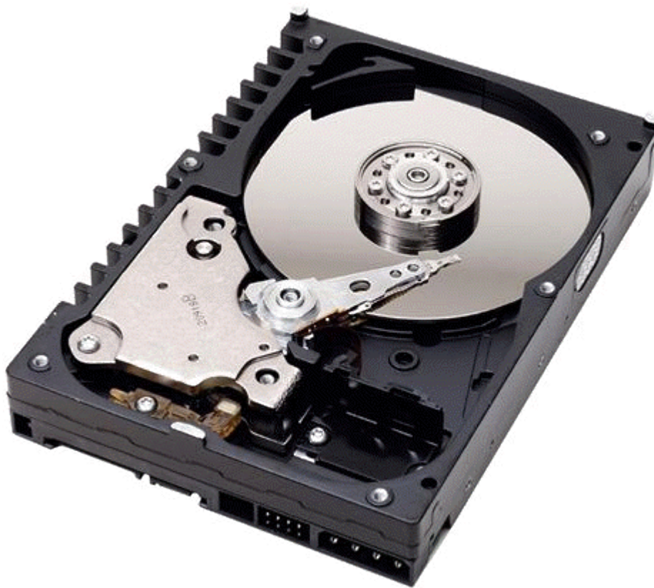
Figure 1.4 A hard disk is a device for permanently storing programs and data.
