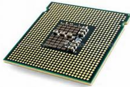
Figure 1.2-1 A CPU must be cooled with a heat sink and a fan. The CPU has a lattice of many pins on its underside.
