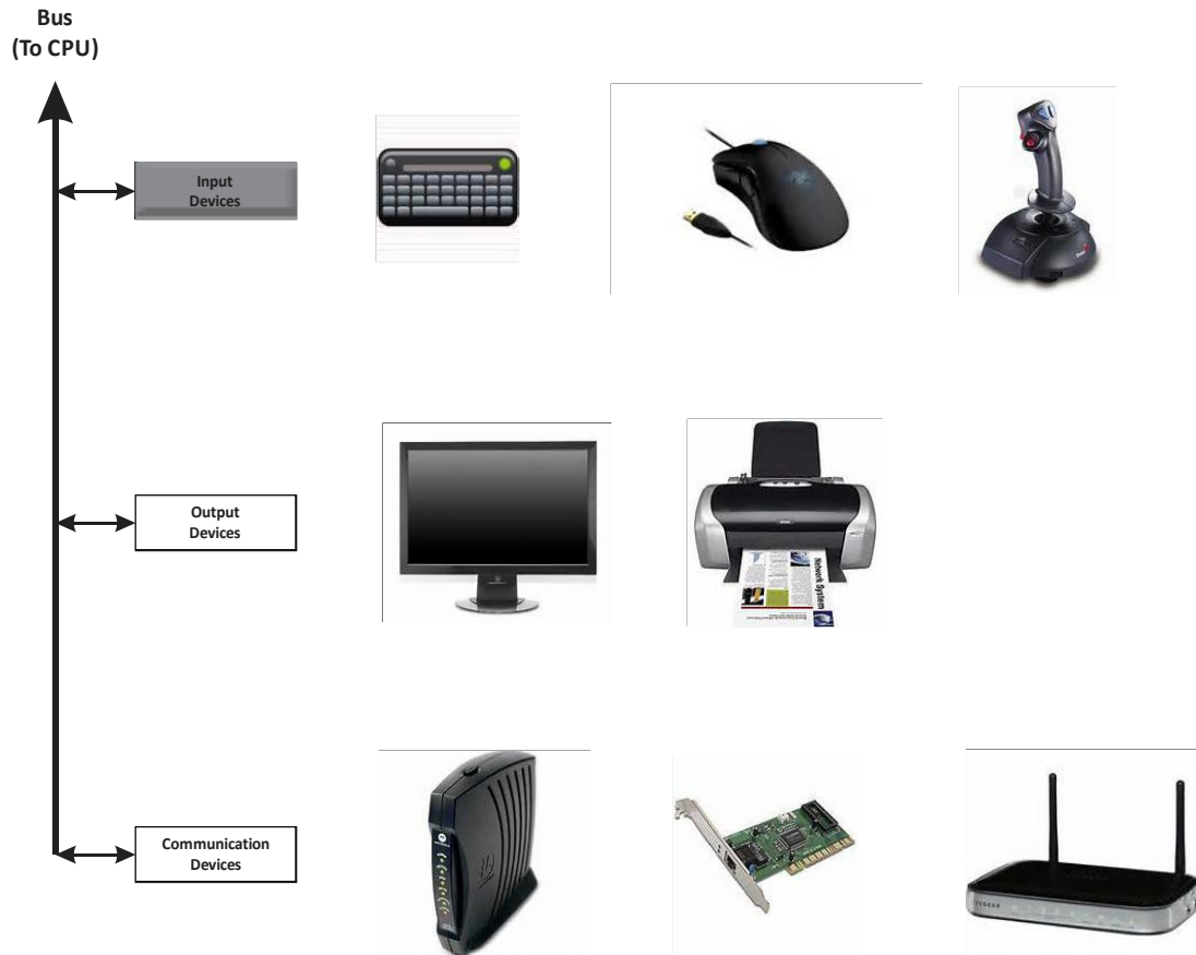
Figure 1.1-2 A computer consists of a CPU, memory, storage devices, input devices, output devices, and communication devices.
