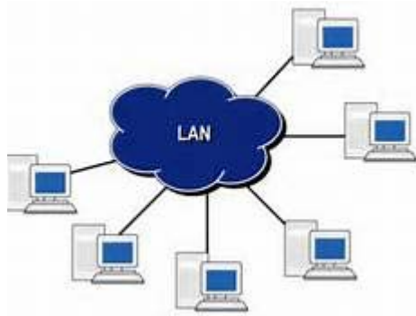
Figure 1.7 A local area network connects computers in close proximity to each other.
